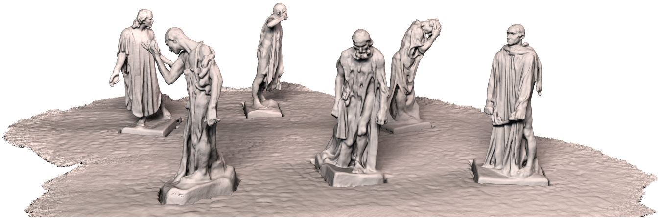
Figure 1: Rodin's "The Burghers of Calais," reconstructed from a stream of images produced by a handheld commodity range camera. The statues are 2 meters tall.
